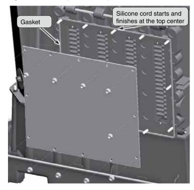
Figure 83 Nut tightening sequence — Ultra-550 Gradually tighten the nuts, repeating the sequence shown below until the torque reaches 160 inch-pounds +/- 10 inch-pounds / 18 N-m +/- 1 N-m
