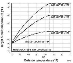
Figure 64 Typical outdoor reset curves
