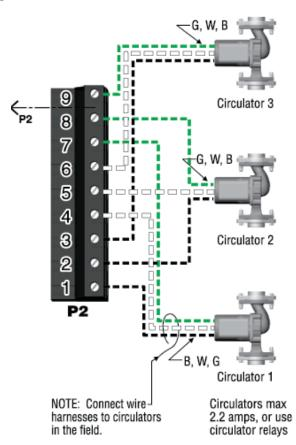
2. You can connect any of the circulators you use to any of the three circulator activation terminals. The U-Control setup allows you to assign which circulators activate on a call for
