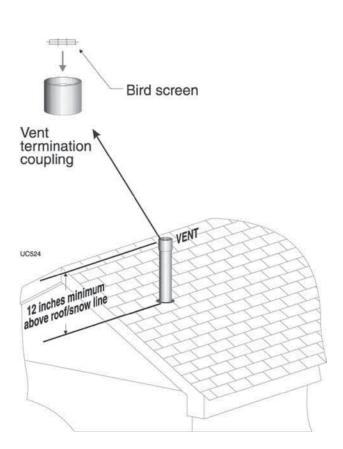
Figure 30 DIRECT EXHAUST — Vertical termination
