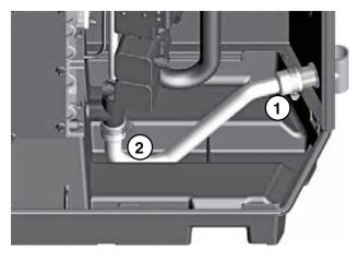
Figure 50 Condensate pump (by others), typical
