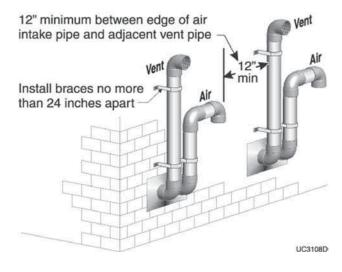
**NOTICE** If the vent/air pipes are extended out beyond the wall, install a coupling at the exit opening, with the coupling butted against the outside plate. Then continue vent/air piping from the coupling.
