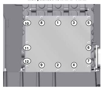
Figure 84 Nut tightening sequence — Ultra-750 Gradually tighten the nuts, repeating the sequence shown below until the torque reaches 160 inch-pounds +/- 10 inch-pounds / 18 N-m +/- 1 N-m
