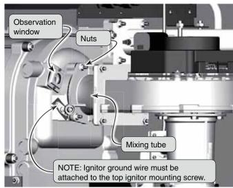
Figure 76 Burner removal and replacement
