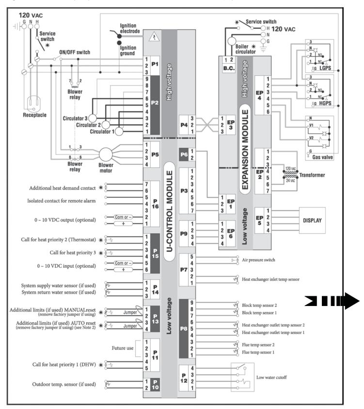
Figure 58 (continued from previous page) Ladder wiring diagram — Ultra-550 & Ultra-750
