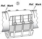
**Note:** If necessary because of flowing water, Steps 3 and 4 can be performed beside the pipe crack or hole. Slide the clamp over the break after the lifter bars have been snapped into place.
