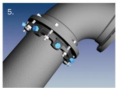
In large sizes (30-48 inch), five or more repetitions may be required. The use of a torque-indicating wrench will facilitate this procedure.
