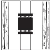
Support pipe and pressure test\* for leaks before concealing joint.
