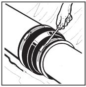
Tighten clamps to 60 inch-lbs. of torque.
