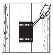
Tighten clamps to 60 inch-lbs. of torque.
