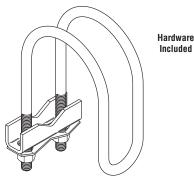
UL Listed Design Load 1" (25mm) thru 4" (100mm) pipe size - 2015 lbs. (8.96kN) Schedule 10 & Schedule 40 Pipe
