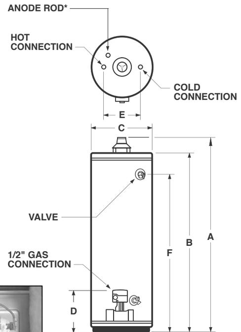
\*Location for optional top-mounted T&P Valve if ordered from factory.
