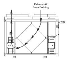
**INSTALLATION** Unit is typically hung by using installation kit supplied with unit. Mounting bolts provided on top four (4) corners of unit.
