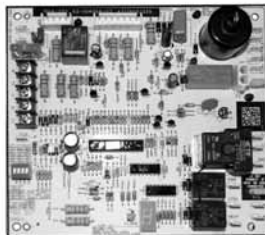
INTEGRATED FURNACE CONTROL
