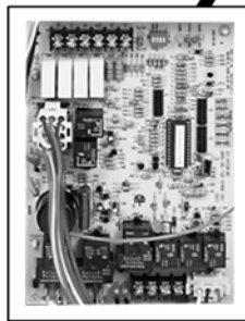
INTEGRATED FURNACE CONTROL
