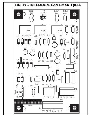
The cooling speed is marked "LOW" on the interface fan board (IFB) (Fig. 17). The factory-shipped settings are noted in Table 4. There are 4 additional speed tap wires available for use in either electric heating or cooling (For color coding on the indoor fan motor leads, see Table 3). The additional 4 speed tap wires are
