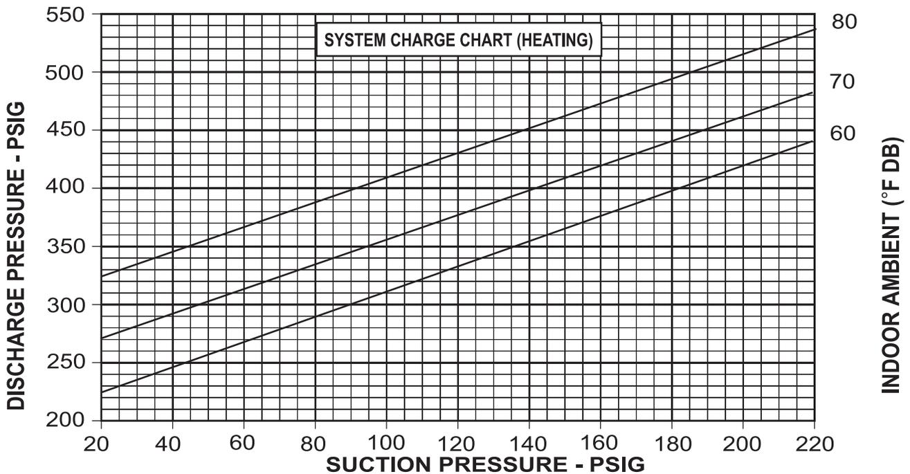
**CAUTION:** BEFORE FINAL REFRIGERANT CHECK, INDOOR RETURN AIR TEMPERATURE MUST BE BETWEEN 72°F & 76°F DB AT 50% R.H. (COOLING), AND NO ICE ON OUTDOOR COILS (HEATING).
