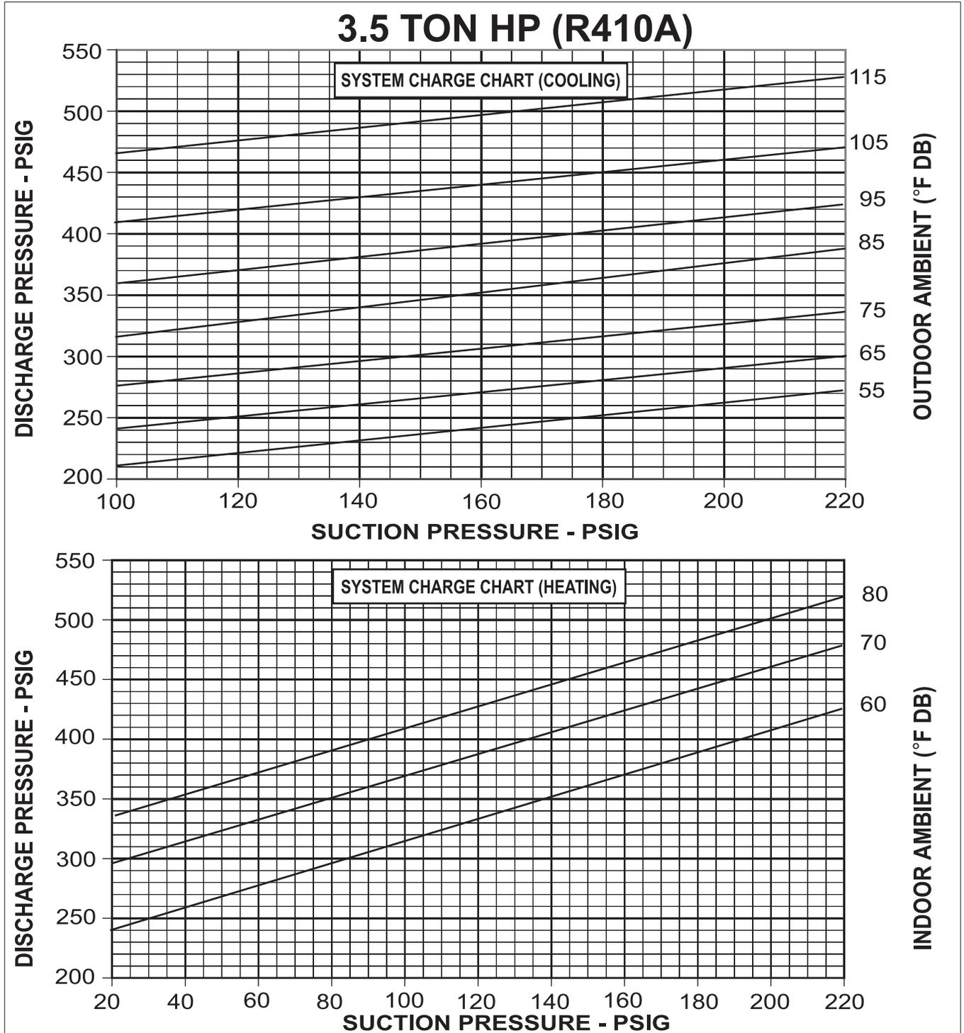
**CAUTION:** BEFORE FINAL REFRIGERANT CHECK, INDOOR RETURN AIR TEMPERATURE MUST BE BETWEEN 72°F & 76°F DB AT 50% R.H. (COOLING), AND NO ICE ON OUTDOOR COILS (HEATING).
