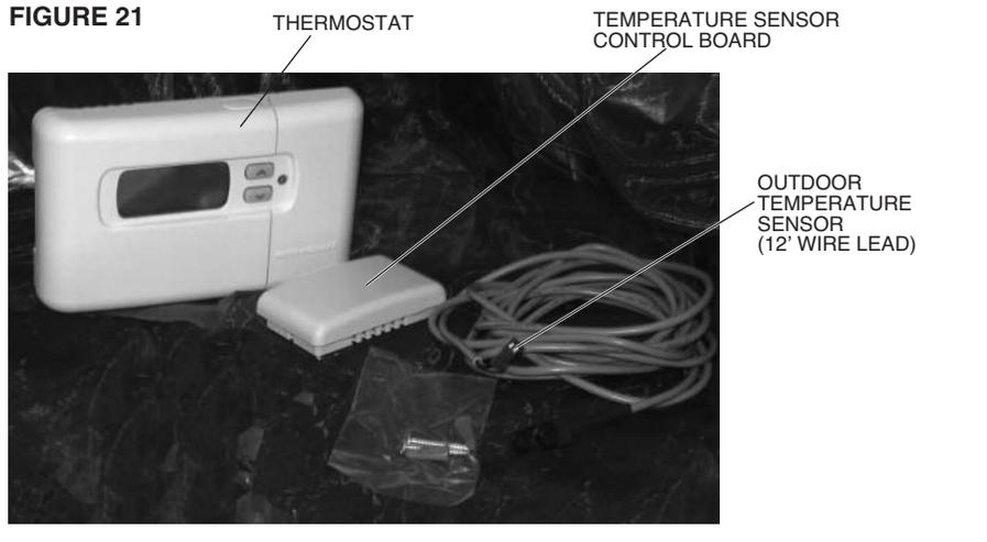
This thermostat requires six (6) wires between the outdoor unit and the thermostat, and another three (3) wires between the thermostat and the outdoor air temperature sensor. Install the room thermostat in accordance with the instruction sheet packed in the box with the thermostat. The low voltage wiring should be sized as shown in Table 7. Run the thermostat lead wires through the "FIELD CONTROL WIRE ENTRANCE" as shown on Figure 1 and connect as shown on the wiring diagram above.
