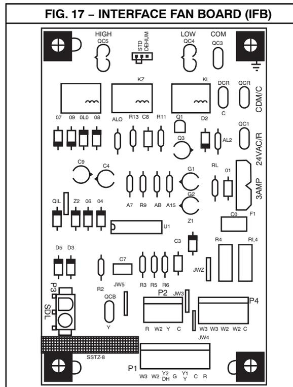
The cooling speed is marked “LOW” on the interface fan board (IFB) (Fig. 17). The factory-shipped settings are noted in Table 4. There are 4 additional speed tap wires available for use in either electric heating or cooling (For color coding on the indoor fan motor leads, see Table 3). The additional 4 speed tap wires are
