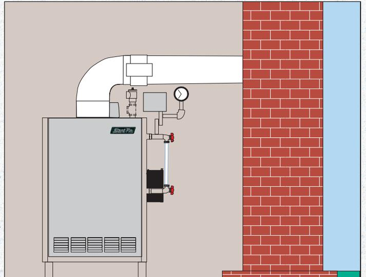
*Clearance requirements of just 18" above the boiler make the GXHA steam model ideal for tight installations.*
