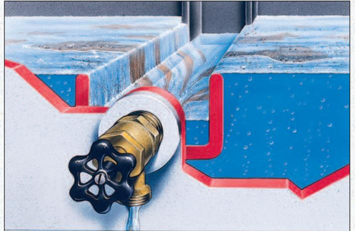
*Built-in speed skimmer trough dramatically reduces steam boiler cleaning time.*
