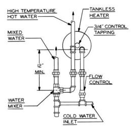
Figure 3.4: Tankless Coil Piping, Water Boiler
