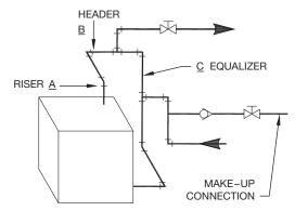
Figure 3.2: Steam Boiler Piping
