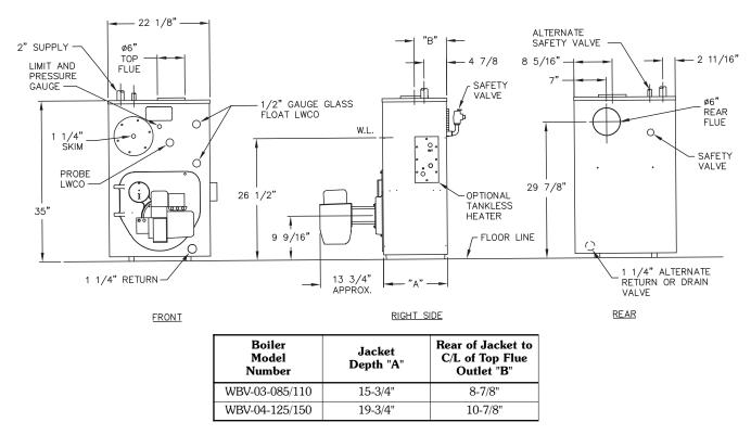
Figure 7.2: Boiler Dimensions, Steam Boiler
