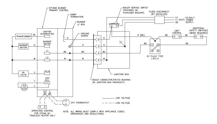
Figure 4.6: Steam with Float Low Water Cut-off
