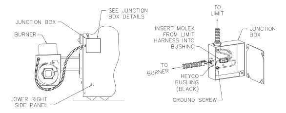
Figure 4.2: Junction Box Wiring, Knockdown Water Boilers
