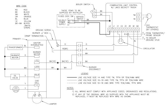
Figure 4.4: Water Boilers, Beckett 7600A Limit Control
