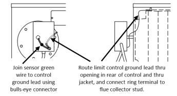
Figure 4.1: Connecting Ground Wire on Beckett Limit Control
