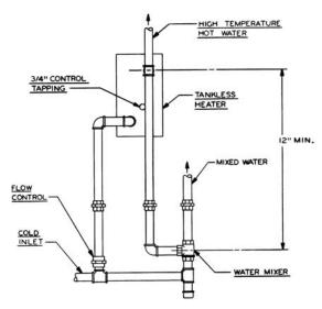
Figure 3.3: Tankless Coil Piping, Steam Boiler
