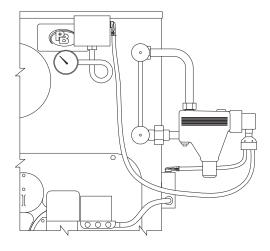
Figure 3.7: Float Low Water Cut-off
