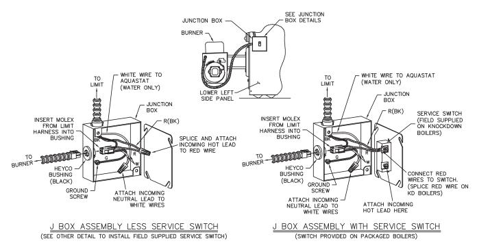
Figure 4.3: Junction Box Wiring, Steam Boilers
