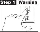
WARNING – To prevent electrical shock or equipment damage, power must be off during installation or servicing of the control. To prevent trol. To prevent
