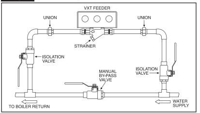
Feeder must be installed with a manual by-pass. Use isolation valves and unions to allow easy removal for service or replacement. Remove and clean the feed valve strainer after the first feed cycle to remove any contaminents introduced during installation.
