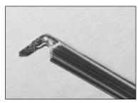
2. Never cut WDCI angle with legs up as chips may fall into the mastic.
