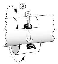
**Note:** If necessary (because of water pressure) Step 4 and Step 5 can be performed beside the pipe break. Slide the clamp over the break after the bolts have been snapped in place.
