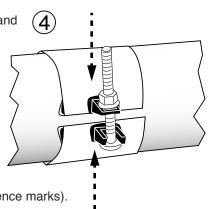
**Step 5** • Starting in the center and working towards each end, tighten all nuts evenly in 20 ft-lb. increments. Keep torques as evenly balanced as possible. Use a wrench with at least a 12" handle.
