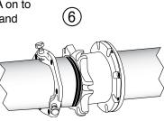
Step 7 • The pipe should be centered such that the space between the OD of the pipe and the ID of the RFCA is even all around the pipe. Slide the RFCA gasket into position with the beveled edge engaging the beveled end of the RFCA body.
