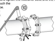
**NOTE:** Do not turn a bolt more than one turn before alternating to the next bolt.
