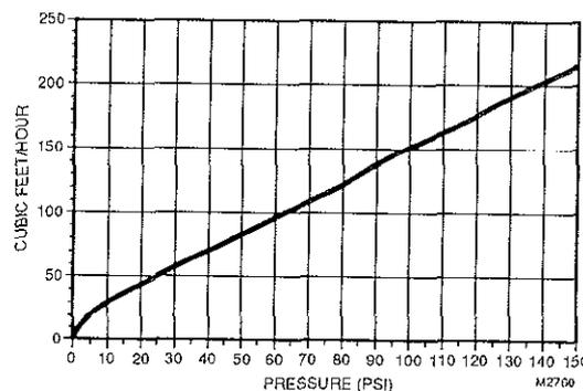
NOTE: Capacity indicated is for device with leakage guard cap correctly installed and operational. Additional capacity may be obtained by removing the leakage guard cap and installing a connection between the vent discharge and drain using Q122A1001 Safe Waste Connector.
