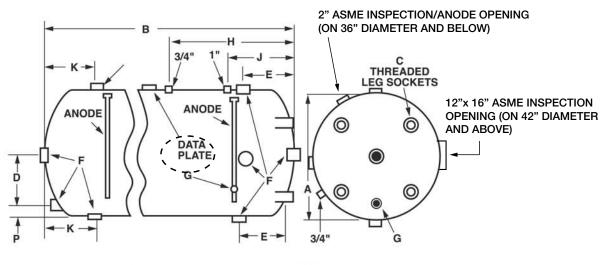
FIGURE 2 - T-140 THRU T-1000A TL-500 - HORIZONTAL MOUNTING ONLY. NO LEG SOCKETS.
