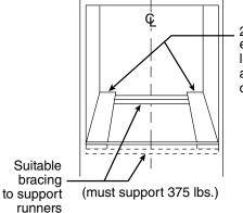
level with bottom of cutout and flush with sides of cutout or solid bottom floor.
