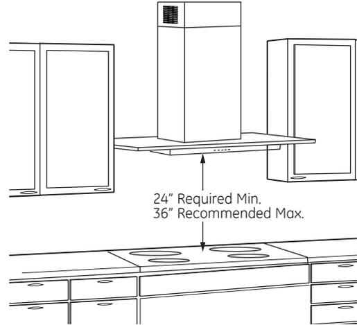
The vent hood must be installed between the 24" required minimum and 36" recommended maximum above the cooking surface. The hood installation height above the cooking surface depends upon ceiling height and duct cover limitations. The telescopic duct cover conceals the ductwork running from the top of the hood to the ceiling. For supplied duct cover ceiling heights, see table on page 5.
