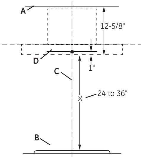
3. Align the top edge of the mounting bracket with the horizontal line (A). Align the center notches of the bracket with the centerline (C) and mark the center of the bracket holes. Remove the bracket to drill the 2 canopy mounting anchors into the wall at the markings. Place the mounting bracket back on the wall and install the 2 mounting screws with 2 washers into the anchors. Tighten screws.
