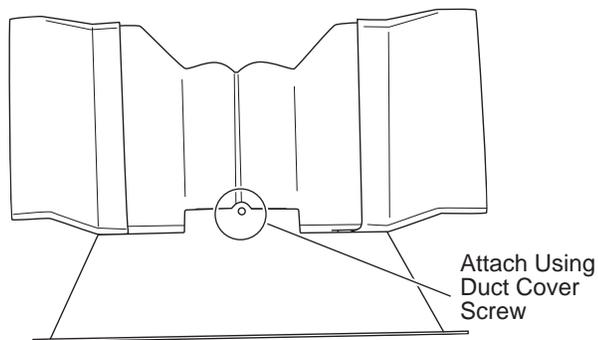
3. Fit the recirculation duct with extensions over the vent exhaust outlet and push down to seat on outlet. Attach the vertical duct work to the top of the hood. Check that the recirculation duct is in the proper orientation (hole facing towards the back of the hood).
