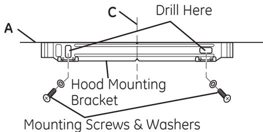
4. Draw a second horizontal line (D) that is 1" added from the (X) distance. Drill a hole into the wall with a 9/32" drill bit at the intersection of the horizontal line (D) and vertical centerline (C). Insert a duct cover anchor.
