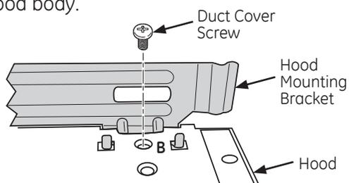
2. Place a mounting screw into the duct cover anchor at the center slot provided on the bottom of the back side of the hood. Securely tighten.
