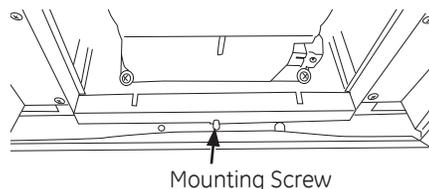
3. Secure the hood to the mounting bracket by fastening a duct cover screw in hole (B) on both sides of bracket shown previously
