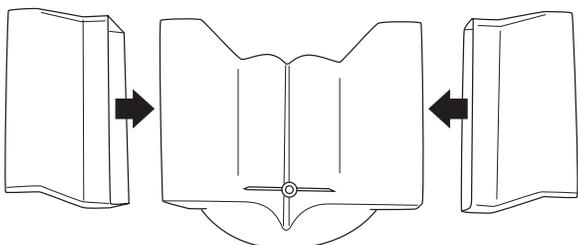
2. Attach the recirculation duct mounting bracket to the recirculation duct using the duct cover screw supplied with the hardware package.
