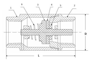
**Specifications:** Designed for residential, commercial or industrial use with water, oil or gas. Threaded ends comply with ANSI B1.20.1. Valve pressure is < 1 PSIG.
