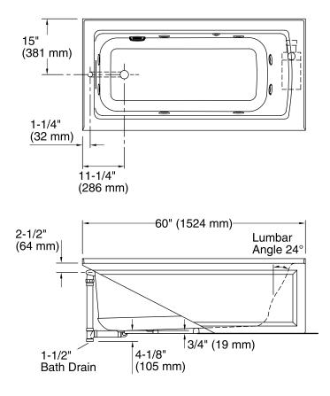
No change in measurements if connected with drain illustrated. (K-7272)
