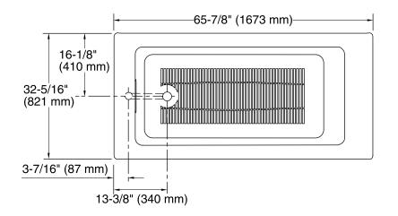
No change in measurements if connected with drain illustrated. (K-7271 or K-7272)
