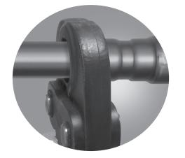
2 Upon identification, use the Viega MegaPress tool to press the fitting, making a permanent leak-proof connection.
