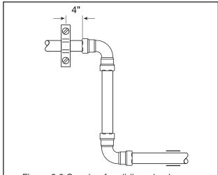
Figure 3.8 Spacing for sliding pipe hanger
