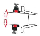
**ONE-LOK's** unique **CAM ACTION** allows the restraining lugs to "rock" and grip the PVC pipe wall more securely as thrust force increases, and allows for subsidence, seismic or other forces after installation, up to the maximum allowed deflection.
