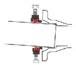
ONE-LOK's cam action also accommodates deflection of the joint during installation, and also allows for subsidence, seismic or other forces after installation, up to the maximum allowed deflection.
