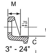
Wedges are ductile iron and heat treated to a hardness of 370 BHN minimum.
