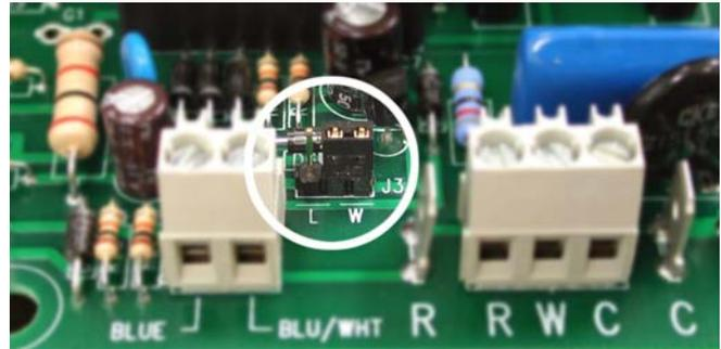
**WARNING:** This shorting device must be in one of the two positions for the circulator pump to properly operate.
