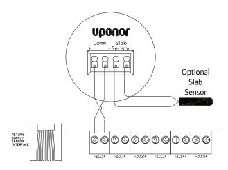
Figure 3: Wall sensor connection to slab sensor
