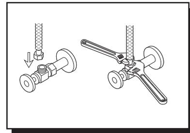
4. Connect and tighten the water supply line nuts by using two adjustable wrenches (avoid twisting or kinking).
