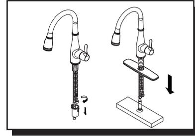
2. Remove lock nut install faucet through center hole.
