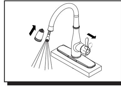
7. After installing faucet, remove aerator and turn on water to remove any left over debris. Re-assemble aerator.
