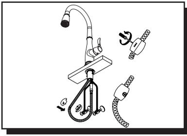
6. Locate lowest point of the hose on the spout side and attach rubber weight.
