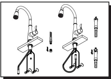
5. Remove the plastic seal cover from the outlet port prior to pushing the hose adapter onto the same port, you will hear a "click" sound once they are joined.
