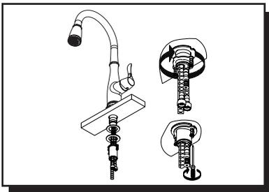
3. Unscrew screws on lock nut. Slide rubber washer and metal washer onto shank. Secure shank with lock nut.
