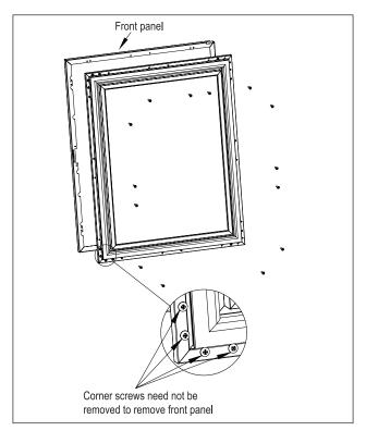
Figure 11. Removing Front Panel
