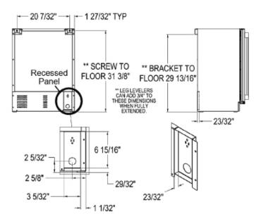
Figure 1. HH (Sottile Model) Electrical Connections
