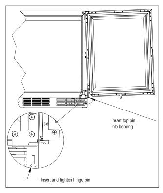
Figure 16. Installing Door
