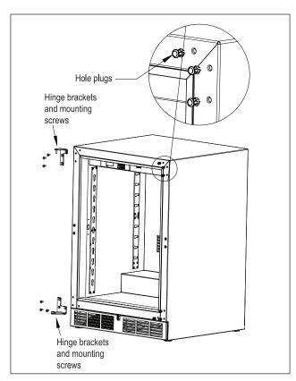
Figure 8. Hinge Removal
