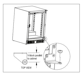
Figure 15. Installing V-Block
