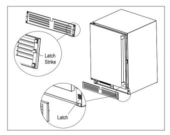
Figure 5. Toe Plate Installation
