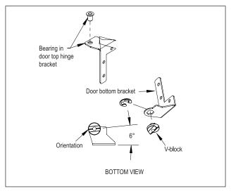
Figure 13. Bearing and V-Block
