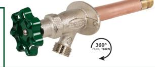
PRIER C-134 provides a year round source of water to areas of structures that are subject to freezing temperatures. The hydrant valve is connected to the supply piping in the heated portion of the structure, eliminating the possibility of freezing. Ordering the C-234 gives you the same style hydrant but with a vandal proof extended lockshield with operating key.
