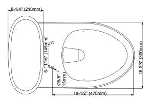
Note: All dimensions and specifications are nominal and may vary: Dimensions of 8'' and greater have a tolerances of +3%. Dimensions less than 8'' have a tolerances of +5%.
