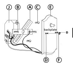
\*\*\* The construction of this fixture will be accomplished by first mounting the mounting strap to the junction box, making all necessary electrical connections, mounting the fixture to the wall and then installing the fixture glass.
