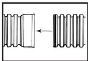
Note: It is recommended that one always lay pipe starting at the down stream end, pushing spigots into bells with the bells facing upstream. Always push spigot ends into bell, **not** bell end into spigot.
