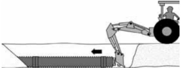
*NOTE: This method requires use of installation stub. DO NOT push backhoe directly against pipe.*
