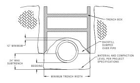
In installations not involving a subtrench, dragging a trench box should only be done if it does not damage the pipe or disrupt the backfill; otherwise, the box should be lifted vertically into its new position, again taking great care not to disturb the pipe or backfill.
