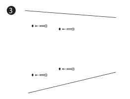
Insert the provided plastic anchors into the drilled holes.
