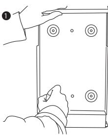
Position the dispenser against the desired spot on the wall where it will be mounted. Use a marker to mark the position of the outside four holes where the holes should be drilled. A spirit level should be used to make sure the dispenser hangs straight.
