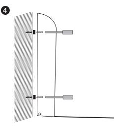
Insert the provided 1.4" inch screws through the dispenser into the provided black rubber distance holders which are placed between the wall and dispenser. Screw the dispenser into position.
