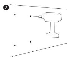
Drill the holes with a 6mm drill bit, a minimum of 1" inch deep.
