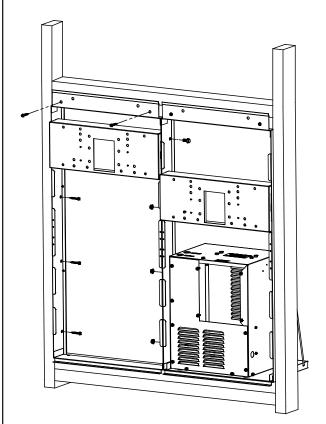
Typical current installation with fountains and panels removed. Disassemble current Bi-Level Refrigerated fountain installation
