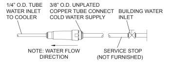
Figure 11 – Water Supply Connections
