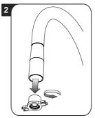
Before removing the aerator make sure that the faucet is turned off. Unscrew the aerator using the aerator installtion key (E) included with the faucet. If the aerator is clogged just rinse it with running water. Do not use detergents. Reassemble the aerator by following the instructions in reverse order.
