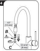
Unscrew the bushing connected to the end of the hose (B) paying attention not to loose the rubber gasket (C).
