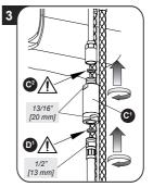
Install the check valve (C2) to the outlet hose with a rubber washer (C1) Secure with wrench
