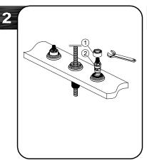
Loosen the cartridge nut (1) and Remove the old cartridge (2) and replace with the new cartridge. Replace the cartridge nut (1).
