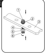
Shut off water supplies. Clean sink or countertop surface. Place flange assembly (2) through the center hole on the sink or contertop(3). Then lock it with rubber washer (4) and metal washer (5) and nut (6). Then place the rubber washer (1) on the flange.
