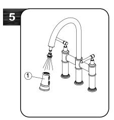
To prevent damage to the internal parts of your faucet from debris that may have collected in the water lines, it will be necessary to flush the faucet. Remove spray head (1). Turn on hot and cold water supplies. Flush water lines for one minute. Reinstall the spray head tightly.
