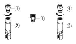
The faucet ships with a 1.5GPM aerator installed. An optional 2.2 GPM aerator is also included in the box. To switch the flow rate of the faucet:
