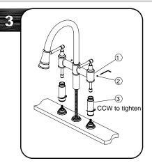
Turn the tubes (3) counterclockwise and reinstall the faucet(1). Tighten the screw (2). Do not overtighten.
