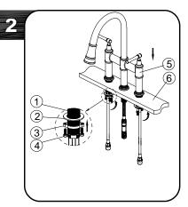
Place new faucet (5) through the three holes in top of sink or countertop (6). From underside, assemble metal washer (2) and nut (3) onto valve body (1) and tighten nut (3). and then tighten the screws (4). Do the same on the opposite side. Do not overtighten.
