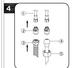
Make connections to water lines with 3/8" female compression supply hoses(1).
