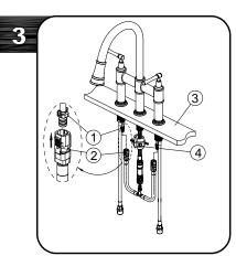
From underneath the sink or countertop (3), align block (1) and tabs (2) on Quick connects. Push Quick connect housing firmly upward and snap onto receiving block. Pull down moderately to ensure connection has been made. If it is necessary to remove quick connect, squeeze tabs on hose between index finger and thumb, then pull down to disconnect. After connecting the hose, install the weight (4) at the lowest point of the hose.
