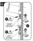
Install the check valve (C1) to the outlet hose with a rubber washer (C2) Secure with wrench
