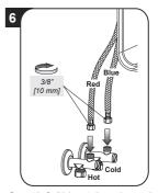
Connect the flexible hoses to the supply connections with rubber gaskets Secure with wrench
