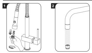
Before removing the aerator make sure that the faucet is turned off. If the supply is not fluid unscrew manually the aerator-holder, remove the filter without damaging and/or loosing the gasket. If the aerator is clogged just rinse it with running water. Do not use detergents. Reassemble the aerator by following the instructions in reverse order.
