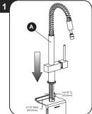
Before inserting the single lever group in the hole of the sink, make sure that the base gasket is properly positioned in its seat and that the flexible hoses are well tightened to the body of the tap. Place the single lever group in the hole of the sink,
