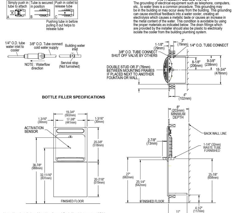
Note : New Installations Must Use Ground Fault Circuit Interrupter (GFCI).
