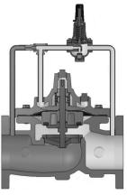
Full Open Operation Using a three way pilot control, pressure relief (typically to atmosphere) can be controlled to the cover that enables the inlet pressure to open the main valve.
