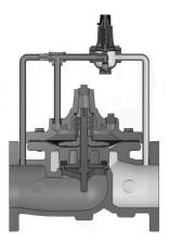
Drip Tight Closing Operation With the use of a three way pilot control, inlet pressure is directed to the cover where the pressure forces the valve closed.
