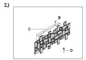
Step 2. Install fixture (C) to wall by tightening machine screws (B) so that back-plate meets the wall. Insert G9 bulbs (D) provided.
