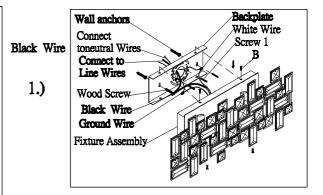
Step 1. Remove mounting bracket (A) from fixture and install it to electrical box. Wire fixture to wires in outlet box. Green wire is for ground.
