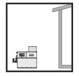
DUCTED AIR w/SIDEWALL INLET
