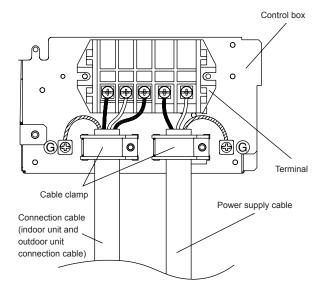
Keep the earth wire longer than the other wires.
