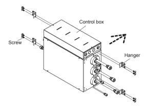
(2) For temporary mounting of the unit, install 2 of the Ø 4×25 screws in the wall, allowing the space of 5~10mm (3/16~3/8 inch) between the wall and the screw heads. Then hook the unit over these 2 screws.
