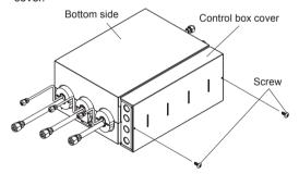
(4) Remove the screws (4 pieces) to remove the bottom panel.
