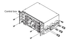
(9) Attach the control box cover and secure it with the screws (2 places).
