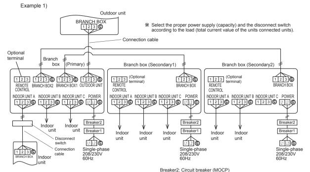
Breaker1: Earth leakage breaker
