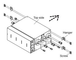
(2) For temporary mounting of the unit, install 2 of the Ø 4×25 screws in the wall, allowing the space of 5~10mm (3/16~3/8 inch) between the wall and the screw heads. Then hook the unit over these 2 screws.
