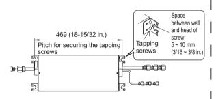
(3) After checking that the unit is flat, secure and mount the branch box with the 8 screws (Ø 4 x 25, accessories) provided including the tapping screws. (The unit's slope must be within ±5° in all directions.)
