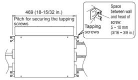
(3) After checking that the unit is flat, secure and mount the branch box with the 8 screws (Ø 4 x 25, accessories) provided including the tapping screws. (The unit's slope must be within ±5° in all directions.)
