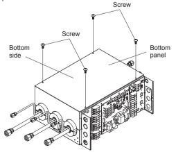
(5) Remove the control box as shown in the figure, and then (6) Attach the control box to the main unit as shown in the change the positioning to the opposite side.
