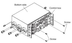
(2) Remove the screws (2 pieces) to remove the control box cover.
