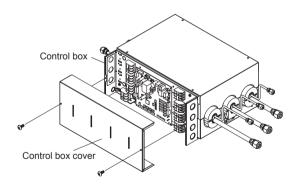
(10) Attach the wiring cover and secure it with the screws (2 places).
