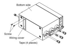
(3) Remove the screws (4 pieces). (Note: Do not remove the control box.)
