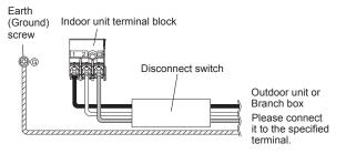
To connect the indoor unit wires to the terminal correctly, refer to the figure for proper Unit: in. (mm) lenath
