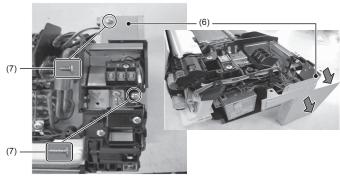
(8) Paste protect seals (2 locations) to prevent the wires from sticking out.
