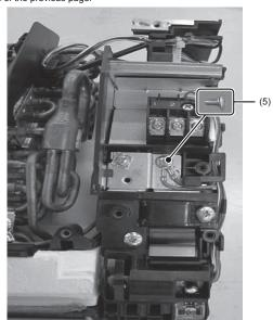
(6) Install the cover of the control box onto the inner side of the rib as shown below.
