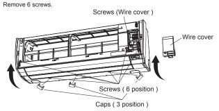
The front panel is pulled to the front, raising the upper surface, and a front panel is removed.
